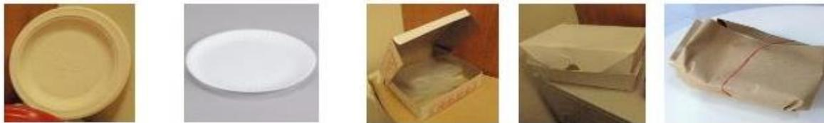
*(From left to right) Corn starch plate; paper plate; paper container with inner plastic sheet, paper container with wax coating; and brown paper wrapping with plastic coating.*
