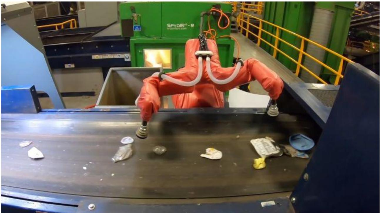
**Bulk Handling Systems Max-AI AQC-C robot**
