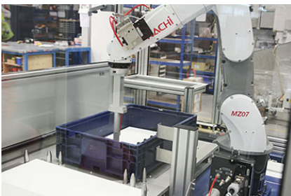
Picture 4 – Robot packs plastic filler caps
