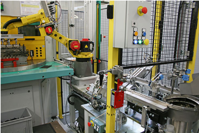
Picture 2 – Six-axis robots load and unload a vertical injection moulding machine and an insert to the moulding
